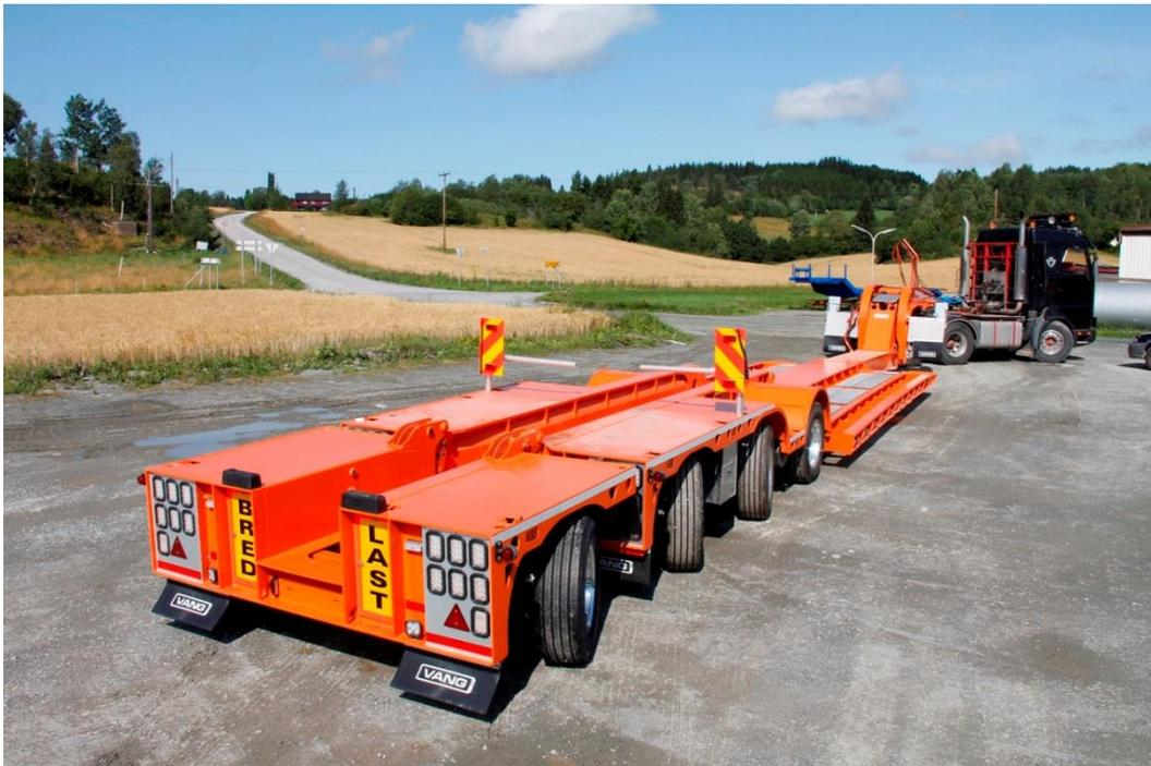
Picture 3: VANGS low bed semitrailer
