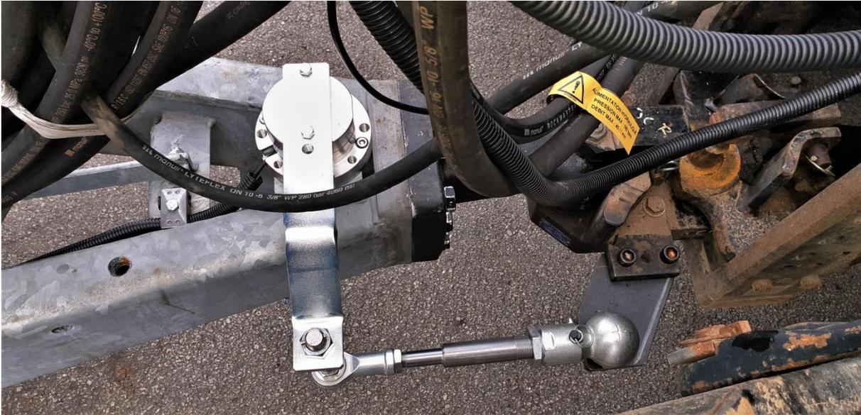
**Figure 1: Stainless steel drawbar encoder with connection to the K50 ball**
