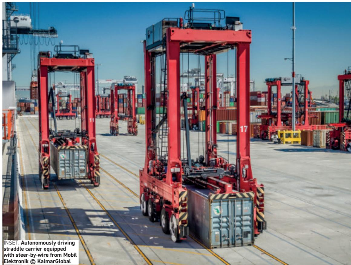
INSET: Autonomously driving straddle carrier equipped with steer-by-wire from Mobil Elektronik © KalmarGlobal
