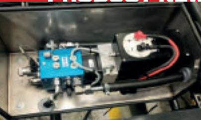
With a 2.3 kW synchronous electric motor, integrated power electronics and a hydraulic pump delivering flows up to 3.43 gpm, Mobil Elektronik's Hydraulic Power Pack can provide electrohydraulic power steering for rear axles in vehicles and equipment.
